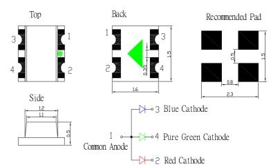
Notes: 1. All dimensions are in millimeters ; 2. Tolerance is  $\pm\,0.10$  mm unless otherwise noted.
